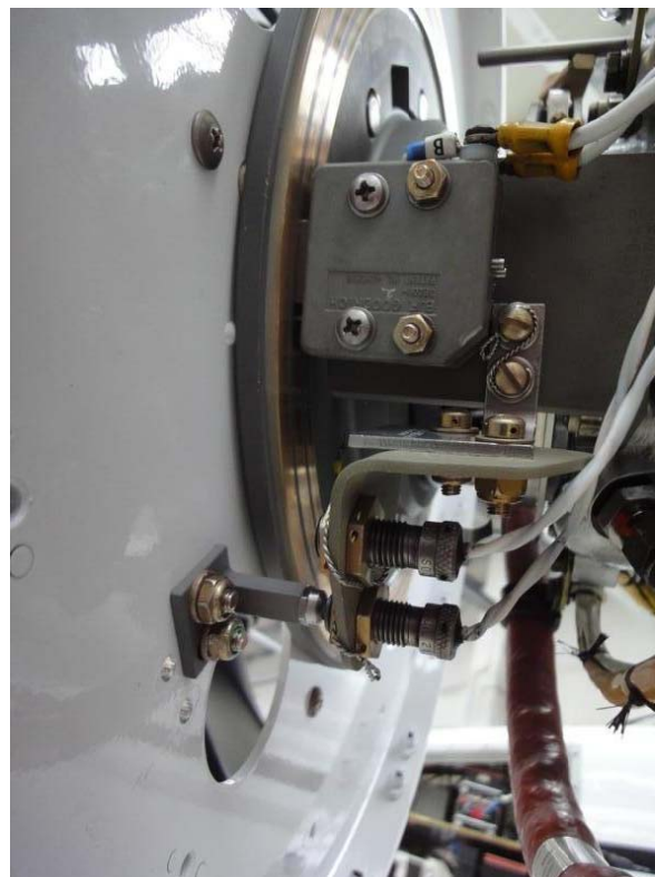
Figure 06 Synchrophaser Bracket 2 (A-1685-4), Magnetic Screw (C-430), preinstalled on the spinner back plate, Sync. Bracket 1 (A-1706-2-( )), preinstalled on the spinner back plate.
